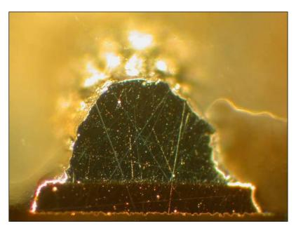
Figure 4 — Cross-section of an acceptable solder joint and surface graping
