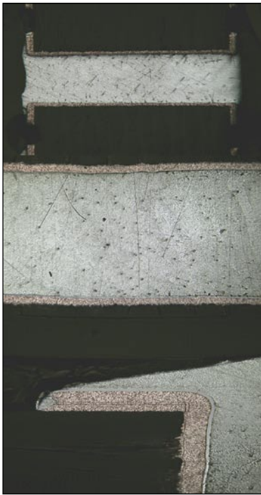
Figure 15 – 28 mil hole in a 62 mil board after thermal shock and thermal stress test
