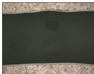
Figure 12 – 10 mil hole in a 93 mil board pulse plated in the bromide bath at 15 ASF with direct agitation (20 x magnification)
