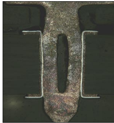
Figure 16 – 62 mil board with a press fit connector pin after the thermal shock test
